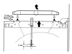
Push the appliance into place. The plug socket necessary for connection of the appliance to the electricity supply should be positioned, so that the plug is not placed in the recess.
